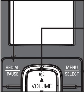
Diagram showing the handset top section with buttons: REDIAL PAUSE, MENU SELECT, and VOLUME. Arrows point from the buttons to the list of functions.
