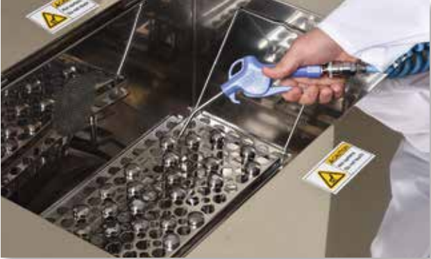
Air wand easily removes excess water
