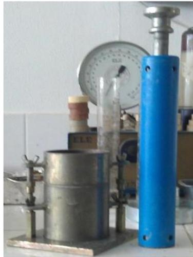
**Figure 3.9:** Proctor compaction test apparatus
