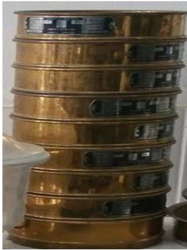
**Figure 3.8:** various sizes of sieves
