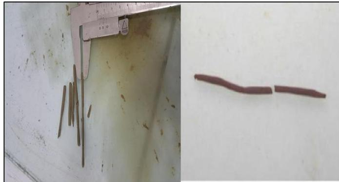
**Figure 3.6:** Determination of plastic limit by crumbling
