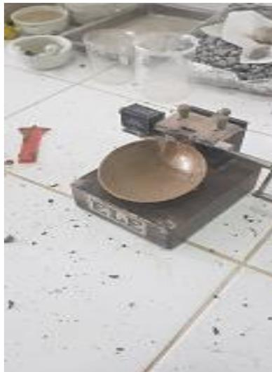
**Figure 3.5:** Liquid limit test apparatus
