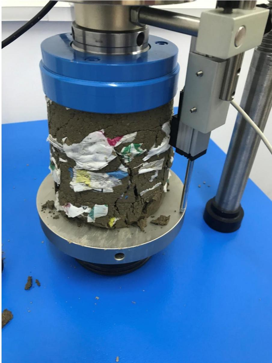
**Figure 4.15:** UCS result showing the failure under stress for 0.4% plastic content
