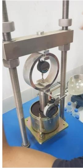
**Figure 3.11:** CBR test apparatus
