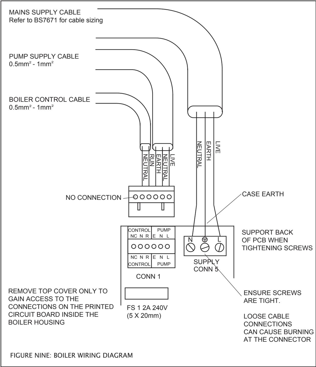
FIGURE NINE: BOILER WIRING DIAGRAM
