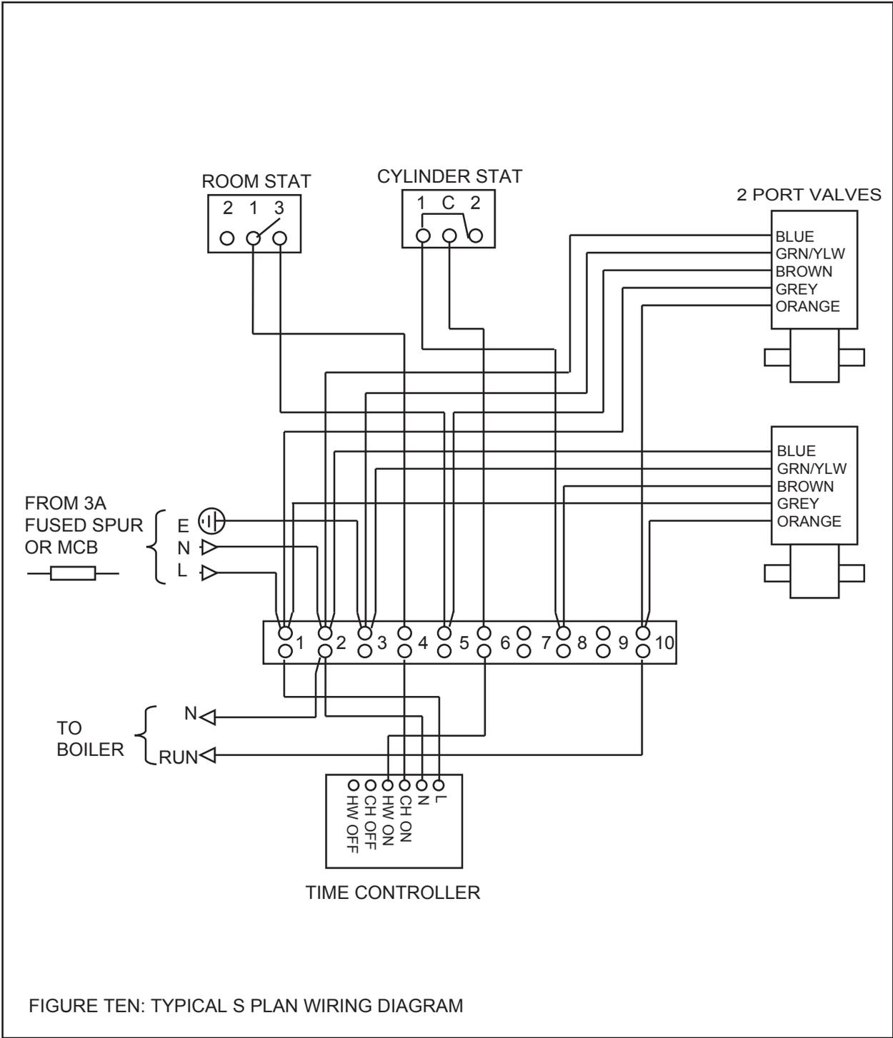
FIGURE TEN: TYPICAL S PLAN WIRING DIAGRAM
