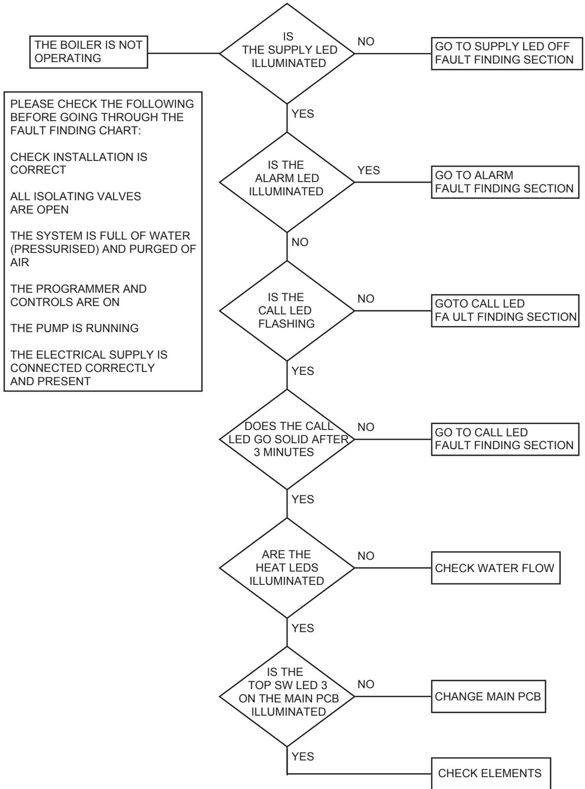
FIGURE SEVENTEEN: FAULT FINDING CHART
