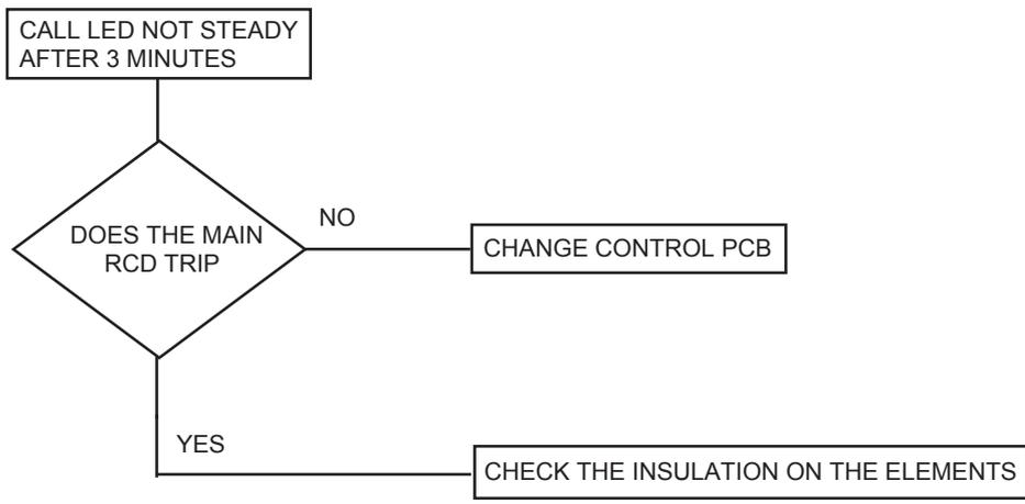
FIGURE TWENTY FOUR: CALL LED NOT STEADY
