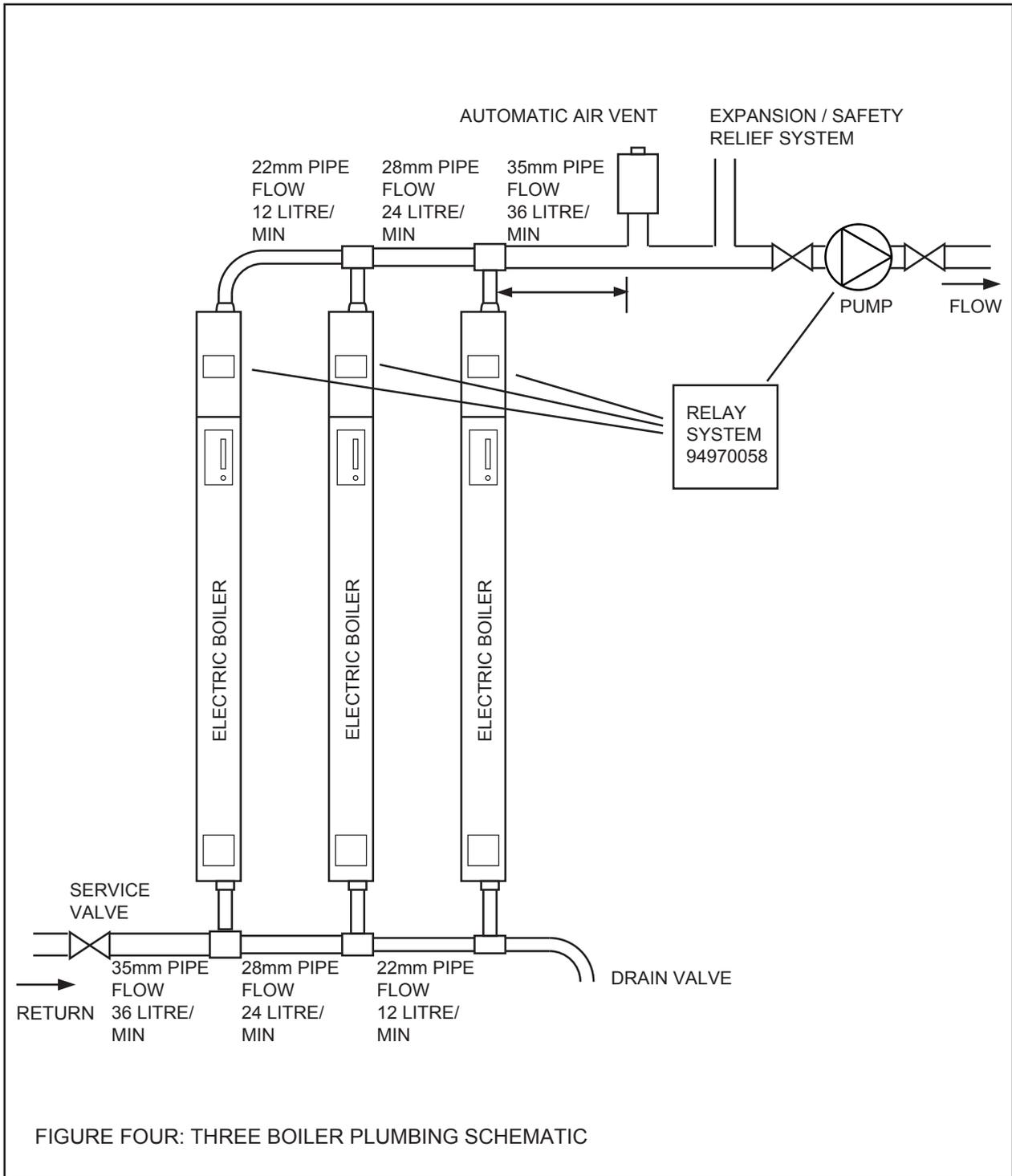
A typical plumbing schematic connecting 3 x 12kW boilers together.
