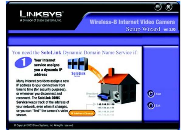
Figure 7-3: SoloLink for Dynamic IP Address
