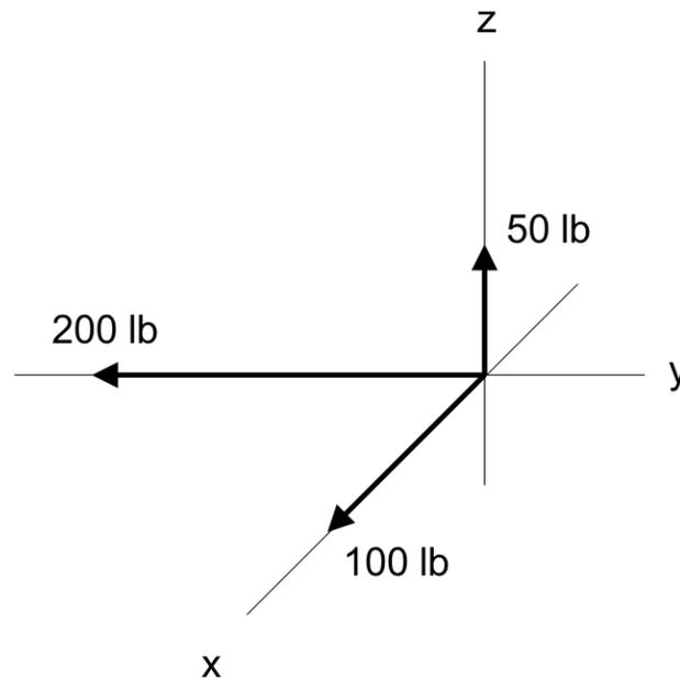
5. Refer to the figure below. Determine the  $x$ ,  $y$ ,  $z$  components of the force  $\mathbf{F}$ . Express the force as a Cartesian vector.
