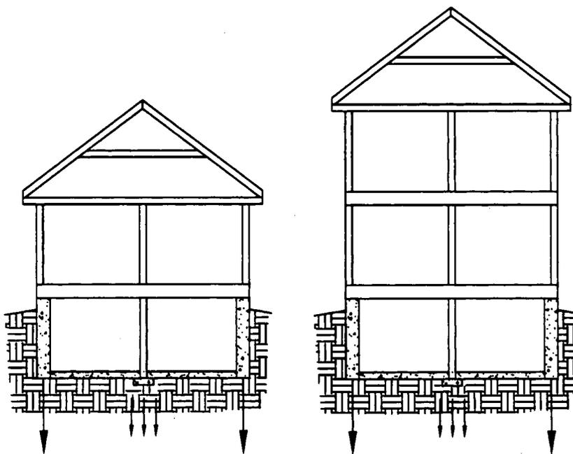
Figure 6. Typical House Sections: Stick-Built Floors & Roof
