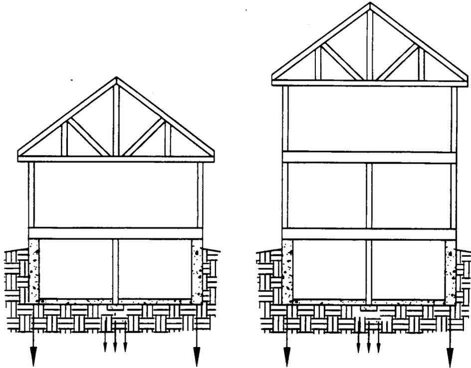
Figure 7. Typical House Sections: Stick-Built Floors with Trussed Roof.
