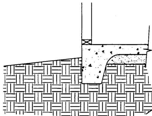
**Figure 5. Slab-on-Grade Construction.**
