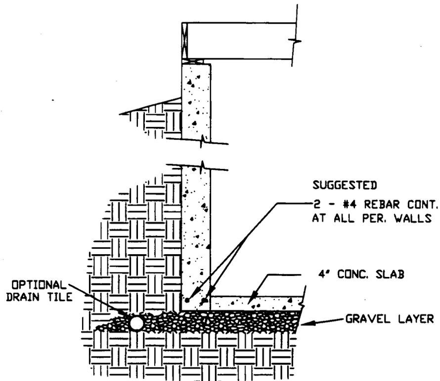
Figure 16. Two- and One-and-One-Half-Story Stemwall Recommendations
