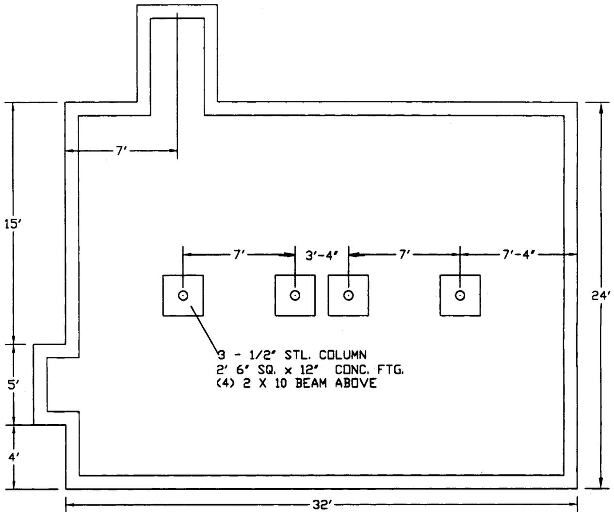
Figure 15. Massachusetts Foundation Plan
