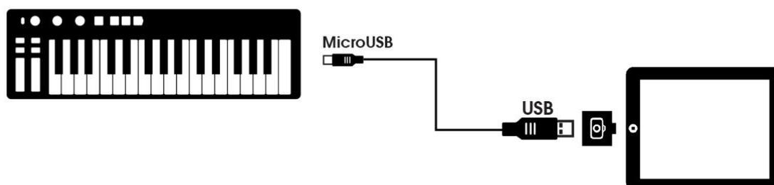
Add a camera connection kit and KeyStep becomes the perfect companion for an iPad. This enables it to be used as a controller for Arturia's iMini, iSem or iProphet applications, for example.
