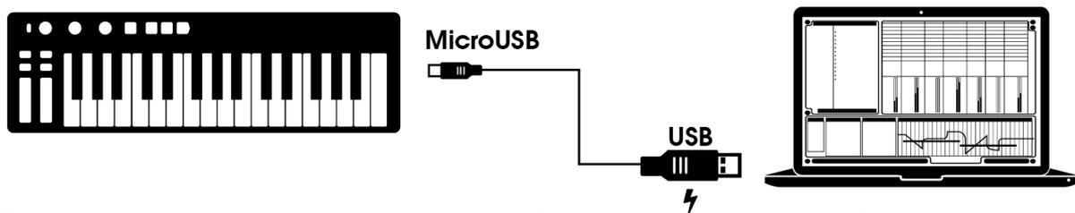
KeyStep is a USB class-compliant controller, so at its most basic level it can be connected to any computer with a USB port and used as an input device for various applications. The included MIDI Control Center software lets you choose which MIDI messages will be sent by the mod strip and pedal, and also enables you to specify the global KeyStep parameters.
