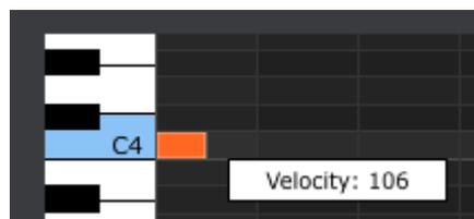
The color of the selected note will change to indicate the velocity value: white is the lowest velocity value and red is the highest velocity value.
