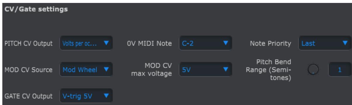
This is where you select the electrical behavior for the Control Voltage connectors.
