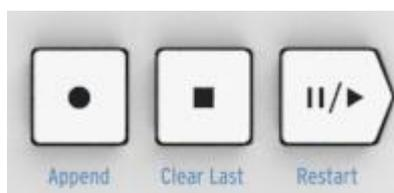
The Transport buttons control the sequencer, the arpeggiator, and external MIDI devices using MIDI Machine Control. But they also can send other MIDI messages if your DAW does not respond to MMC commands. Use the MIDI Control Center to make changes.
