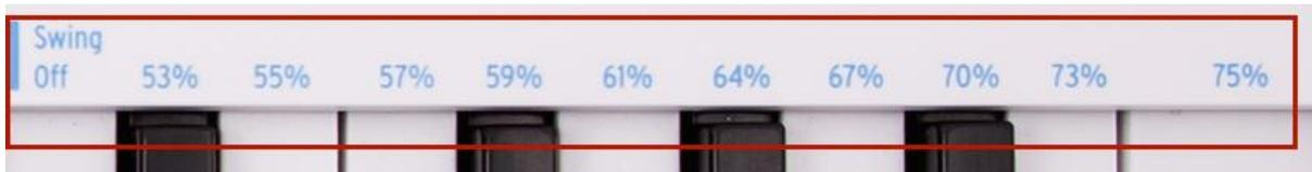
Swing introduces a “shuffle” feel to the active sequence or arpeggio. 11 different settings are available, ranging from Off (no swing, or 50%) through varying degrees of swing amount (53-75%). To make a selection, Hold Shift and press the appropriate key.
