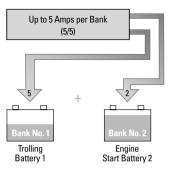
Competitive chargers have an amp limitation per bank. As illustrated the (5/5) 10 amp charger can not transfer the unused 3 amps not required by the engine start battery, leaving only a maximum of 5 amps for the trolling motor battery.
